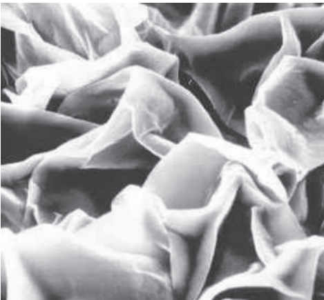
Figure 1 The folding of flat clay particles.
