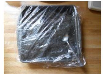
7) Securely cover pan (with sample and water inside) with plastic wrap so the moisture does not escape.
