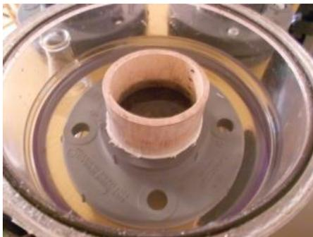
19) Pour distilled water into the top of the Water Holding Mold until there is 2cm of water on top of the sample by pouring from a beaker.
