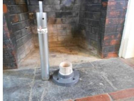
8) Get a clean, dry Water Holding Mold from the **flow bench**. Place a **Whatman #541** filter paper on the bottom inside the mold.
