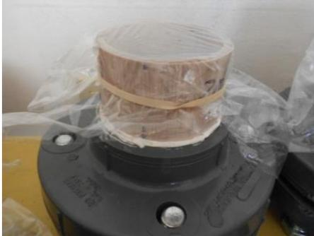
28) Cover the Water Holding Mold with plastic wrap, secure with a rubber band and poke a hole in the top. Make sure to not break the surface of the sample.
