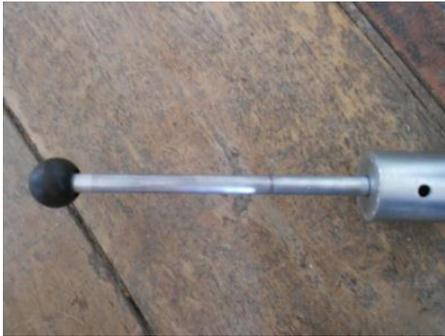
8) Make sure the **10 cm mark** in permanent marker is clearly depicted on compaction hammer. If not, measure 10 cm from the bottom of the hammer handle and make a new mark.
