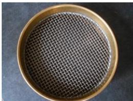
2) If this is the first time the sample is being used remove any large pieces of rubber or knots of fiber by sieving the sample with a **#4 synthetic sieve** and picking
