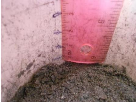
17) Identify height of sample in Water Holding Mold by counting down the centimeter marks on the inside of the Water Holding Mold starting at the top. The first line is 9 cm. If the surface of the sample is compacted between the lines then estimate. Record the sample height on the data sheet.
