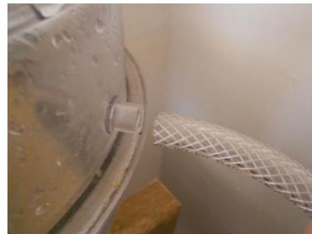
22) Attach the hose from the vacuum pump to the vacuum desiccator lid.
