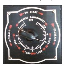
6) When the furnace has reached 800°F to 850°F, turn the dial setting to a setting between "4.6" and "4.8" and press the start button again.
