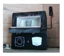
5) Set the muffle furnace to the "8.0" setting during heatup. Press the green start button on the **timer**. It will take approximately 45 - 75 min to reach the desired temperature of 825°F (440°C).
