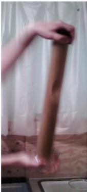
13) Start the timer right after the 60 flips and work quickly to place the sedimentation cylinder into the constant-temperature tank (or on the counter if not using a water bath) and remove the rubber stopper.
