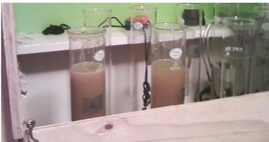
14) Take and record hydrometer readings at time intervals of 1, 2, 5, 15, 30, 60, 250, and 1440 minutes. To take a hydrometer reading, gently place the hydrometer into the top of the sedimentation cylinder so that it is just below the level you expect the reading to be at. Allow the hydrometer to sit for 20 seconds before taking a reading at the top of the meniscus to the nearest 0.1 g/L.
