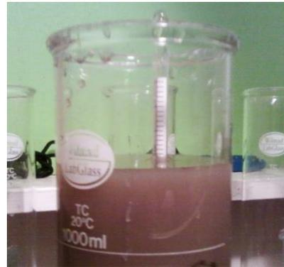
15) After each reading, gently remove the hydrometer and clean by placing it into the cylinder of distilled water and twirling it gently or by spraying it off with distilled water and wiping dry with a paper towel. Then, gently insert a thermometer into the suspension and record the temperature.
