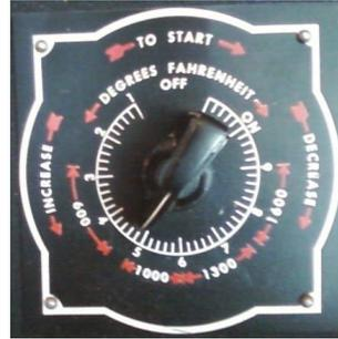
16. *Important notes* 1) Do not let the temperature inside the furnace exceed 900°F. This may cause the sand particles to crack. 2) DO NOT OPEN the muffle furnace while it is operating or the crucibles will undergo thermal shock.
